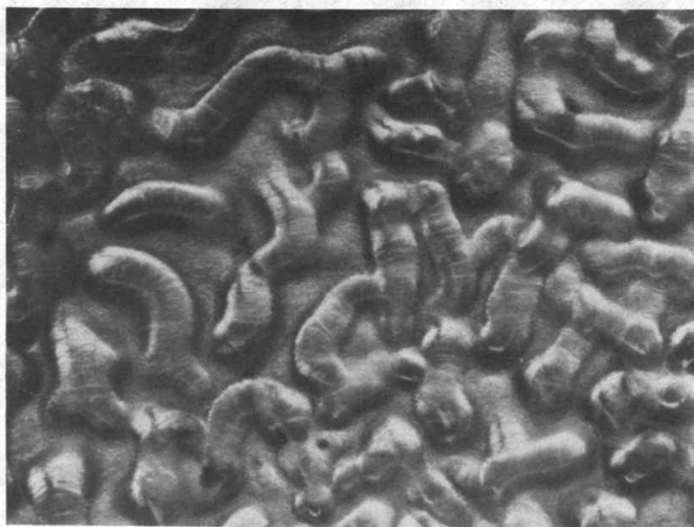
Fig. 4. Optical microphotograph of fibrillar structures observed for PVCA layers at crossed nicols (magnified 180 \times ).
